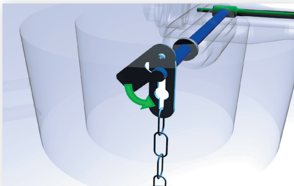
■ Patented displacer hook assembly.
